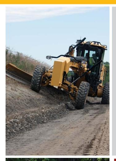
If you work in soft underfoot conditions where traction can be a challenge, optional All Wheel Drive (AWD) can give you the additional power to the ground you need to work more efficiently in mud, gravel, sand or snow. The added traction helps reduce sliding on side slopes.
