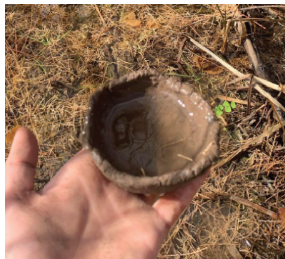
Figure 3: Soil adjacent to standing water in the borrow pit formed into a small bowl that holds water Kari Hackney
