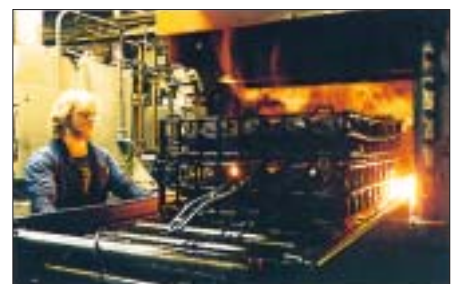
Batch type furnace with a controlled atmosphere
