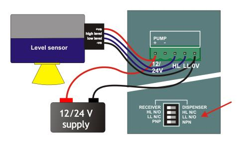
NOTE: The system will function with high level monitoring only. Low level monitoring is used for indication purposes only.
