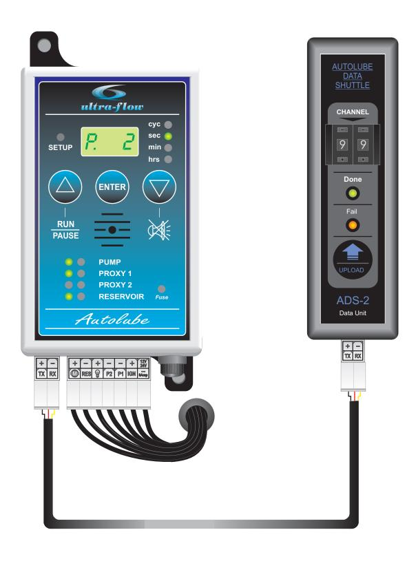
The autolube controller has the capacity to store all critical faults up to 80 records. The Data Shuttle is a device that can retrieve this data without the use of a laptop PC. The data shuttle can retrieve information from up to 100 different controllers. This information can be then downloaded from the Data Shuttle to your desktop PC to the autolube program whereby all the relevant faults can be scrutinized.
