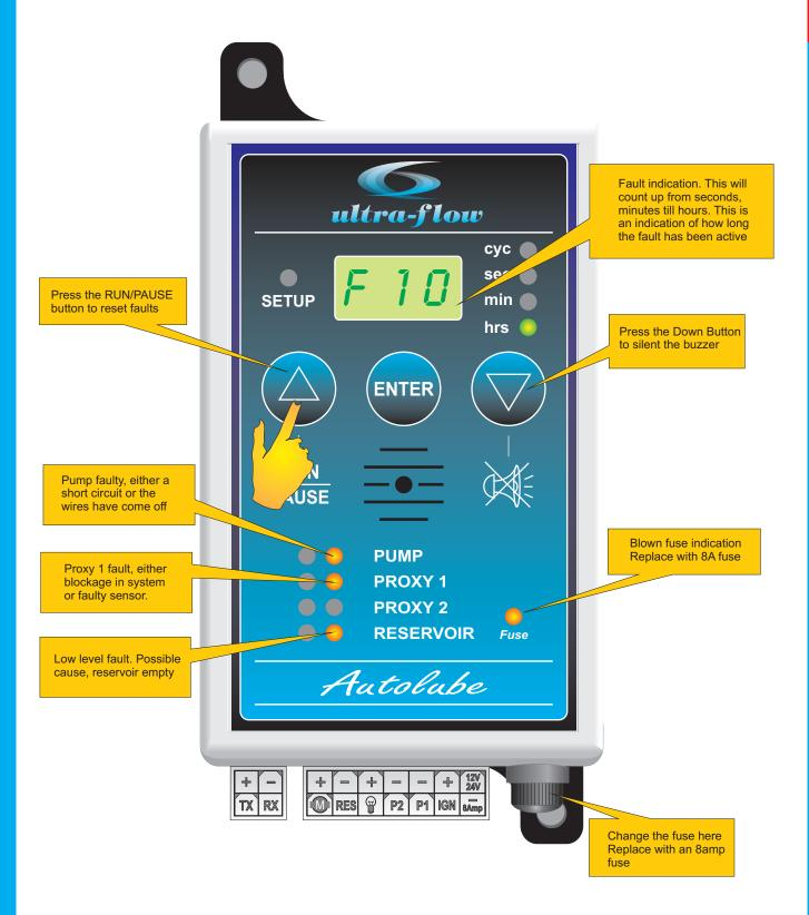
**NOTE**: IN ORDER FOR A FAULT TO BE TOTALLY RESET THE UNIT MUST PERFORM I COMPLETE CYCLE OF RUN AND PAUSE TO CANCEL AN EXISTING FAULT OUT OF MEMORY. THE UNIT IS DESIGNED TO MEMORIZE THE TOTAL TIME OF ANY SPECIFIC FAULT. THE ONLY WAY THE UNIT CAN FUNCTION CORRECTLY WITHOUT THE SAME FAULT OCCURRING IS FOR IT TO RUN 1 COMPLETE CYCLE.
