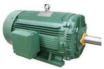
APT NEMA EPACT are three phase induction motors which are single speed, totally enclosed, self-cooled, continuous duty, low voltage and cage type. The motors conform to NEMA MG1 standard and adopt casting iron frames. The efficiency meets America NEMA EPACT standard. Service factor is 1.15. The motors have passed America CC certificate and Canada CSA certificate.
