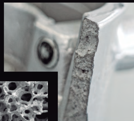
Structure INJECTION ALUMINIUM
