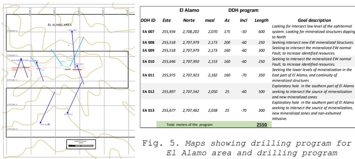
Fig. 5. Maps showing drilling program for El Alamo area and drilling program summary, (in light blue, 2019 diamond holes, in strong blue, proposed hole
