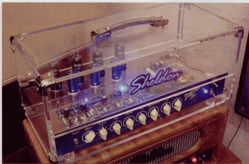
Glass act A spectacular all-perspex TT1 head, able to cope with two or four 6V6 or 6L6 valves
