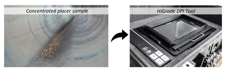
The pan concentrate is placed on a specially designed sample holder from where a high resolution image is created with an optical scanner. Then the automatic HiGrade DPI particle analyzer detects gold particles based on their golden color and calculates the gold grade of the sample. The automatically generated report includes unique statistics on the particle size distribution and particle shape. The analysis takes less than 5 min, requires no consumables and is non-destructive.
