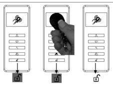
To set/unset the system using the Internal Tag Reader, present a pre-programmed tag to the tag symbol as shown.
