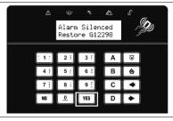
When the time is displayed, enter the number given to you by the ARC. 'Engineer Restore Performed' will be displayed.
