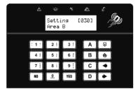
If a final exit input is activated during the setting procedure the system will quick set area A.
