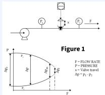
Once the specific gravity (SG) and flow (F) of the fluid are known, the valve's Cv can be calculated once the pressure drop ( $\Delta p$ ) is determined.
