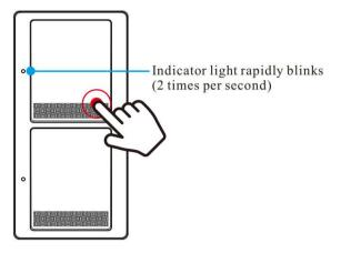
**Step.1**. After powering on, press and hold the ON/OFF button for 5-7 seconds, and the indicator light flashes quickly
