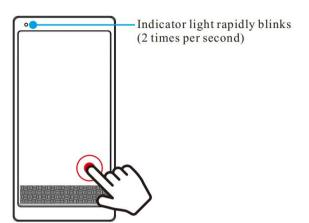
**Step.1**. After powering on, press and hold the ON/OFF button for 5-7 seconds, and the indicator light flashes quickly
