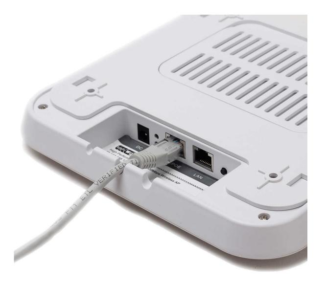
The network cable is connected from the POE switch to the AP (poe) port
