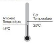
Set temperature > ambient temperature: heating function on. Set temperature ≤ ambient temperature: heating function stops
