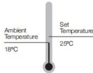
Set temperature > ambient temperature: heating function on.
