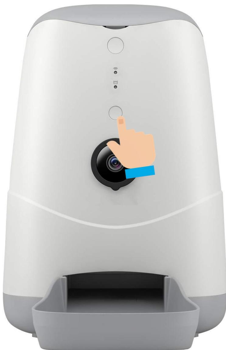
Power on the feeder and wait for the Wi-Fi Indicator start blinking slowly along with a start-up sound. It may take a few minutes. (If not, please long press the Manual Feed Button to reset the device).
