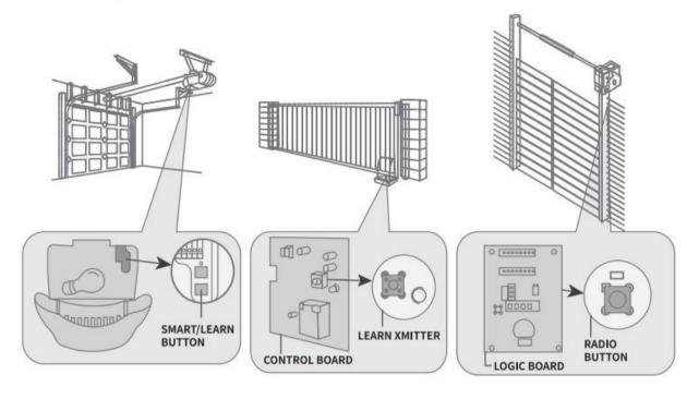
4.Press the ON/OFF button and the Program Led will flash. When the Program Led stops flash, you can then press that button next time, repeat this process multiple times until a click is heard from the garage door opener, or the bulb on the garage door opener blinks, or the garage door opens/closes, or a beep is heard from the door operator.
