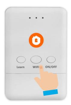
Step2:When The Blue Light Is Always On, Press And Hold the reset button For 5 Seconds
