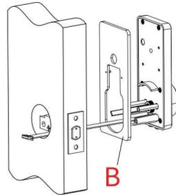
**Step 4** Install mounting plate (C) with M4 cross flat head bolt (G) on the door.
