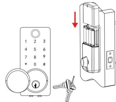
•Testing the lock by rotating the knob on unit D and using mechanical key(J).
