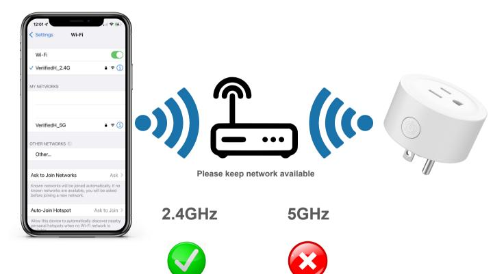
The router supports the 2.4GHz WiFi (doesn't support the 5GHz), and is connected to the WiFi network. Please set the parameters of the router before connecting the WiFi network, and record the SSID and password of your WiFi.
