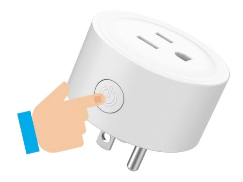
Step2:When The Blue Light Is Always On, Press And Hold The Button For 5 Seconds
