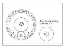
Alarm module > Disable the factory lock by pushing the lever clockwise.
