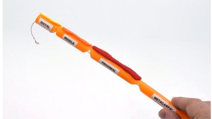
**10** | Hot glue the felt bones to your articulated finger opposite your cut holes, except for the metacarpal, which will be applied a bit later when building the robotic finger.
