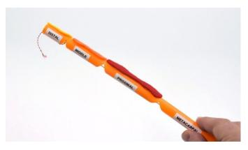
**10** Hot glue the felt bones to your articulated finger opposite your cut holes, except for the metacarpal, which will be applied a bit later when building the robotic finger.
