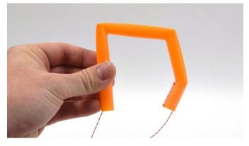
**7** | Check your finger functionality by pulling the thread. The digits should bend progressively and in order, from top to bottom.
