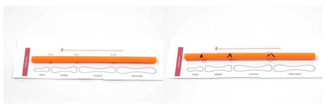
1 | Cut out your template and align straw. Use this2 | Using your spacing guide, mark location of cuts on<br/>template as a stencil for making each articulated finger. the straw.
