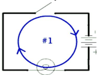
We make electricity by creating an electric circuit. Let's take the case where you are turning on a light in your house: when you flip the switch "on" you are completing the electric circuit and causing electricity and electrons to flow through the light bulb, turning the light "ON."
