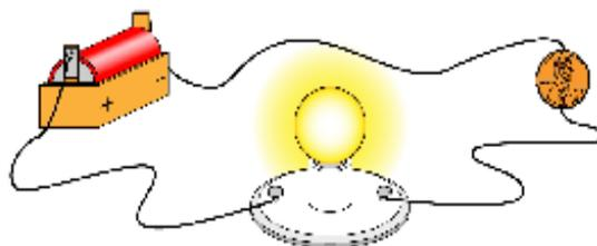
Touch the free ends of the wire to the object you are testing. If the light bulb lights up, the object is made from a conductor. If it does not, the object is made from an insulator.
