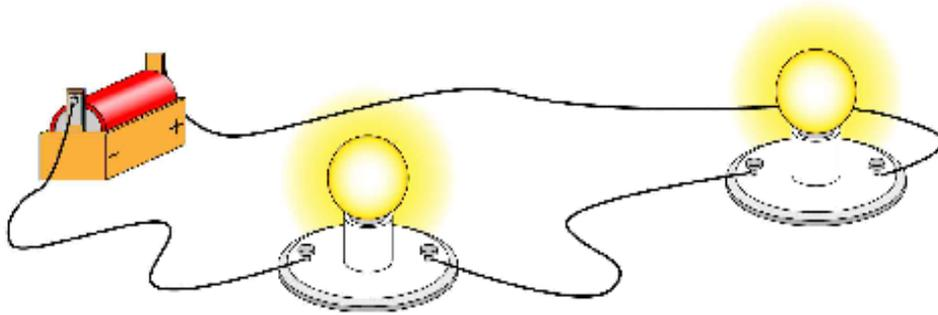
If a light bulb is missing or broken in a series circuit, will the other bulb light? Explain.
