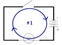
We make electricity by creating an electric circuit. Let's take the case where you are turning on a light in your house: when you flip the switch "on" you are completing the electric circuit and causing electricity and electrons to flow through the light bulb, turning the light "ON."
