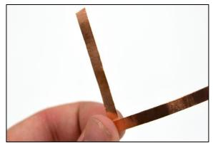
• The key to making successful circuits with copper tape has a lot to with how good the connections are between LEDs, paperclips, and switch contacts with the tape. Folding the tape is the best way to do this rather than laying on multiple strands of tape to make the turn.
