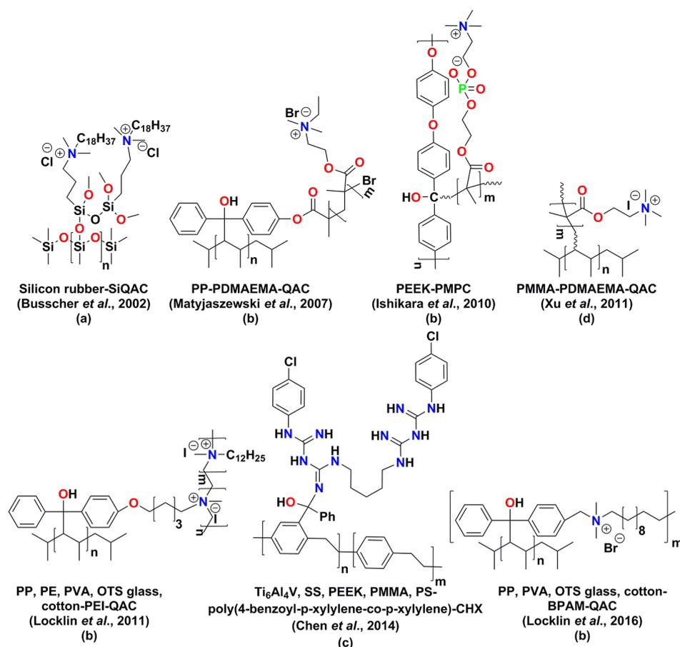
**Figure 1.** Examples from the literature of the covalent functionalization of plastic material surfaces with quaternary ammonium anchored biocides through (a) silane anchors, (b) benzophenone C–H insertions to surfaces or (c) grafting to a biocide, that is, chlorhexidine, CHX, or (d) acrylate photoinitiated by surface immobilized benzophenone.
