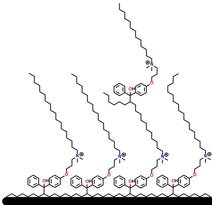
**Figure 4.** Schematic representation of surface grafted branching of **5b** leading to an increase in coating thickness and charge density on a substrate such as PS.
