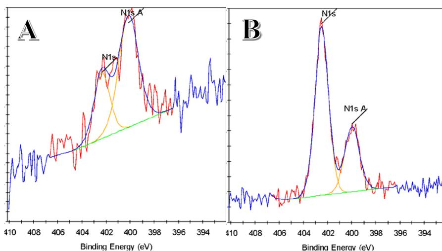
**Figure 6.** XPS data corresponding to the nitrogen content for the control (A) and **5b** coated (B) PS samples.
