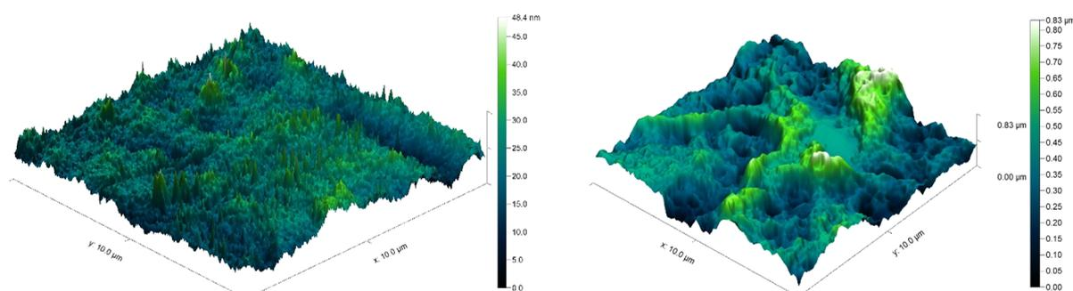
**Figure 5.** AFM images of PS control (left) and  $\times 2$  coating of **5b** on PS (right).
