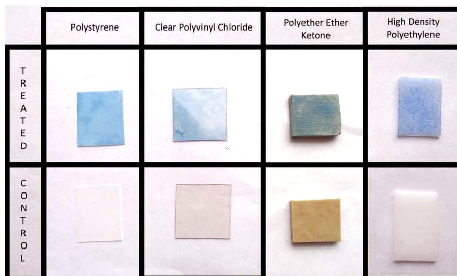
Figure 3. Treated and untreated surfaces stained with bromophenol blue dye.
