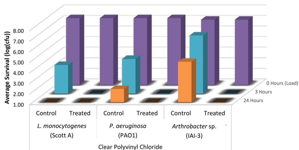
**Figure 8.** Graph depicting the average survival of *L. monocytogenes*, *P. aeruginosa*, and *Arthrobacter sp.*, when inoculated onto QAC-treated (**5b**) and control samples of CPVC.
