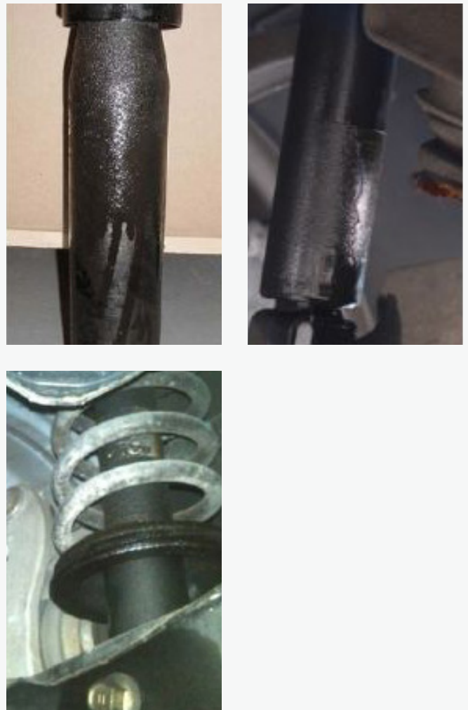
Figure 4.5 Examples of leaking shock absorbers
