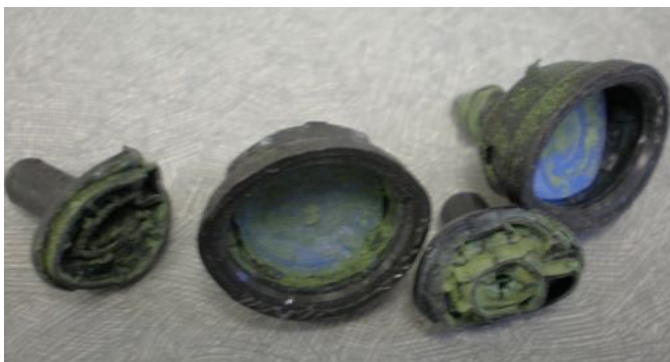
Biofilm clogged pressure compensating emitters
