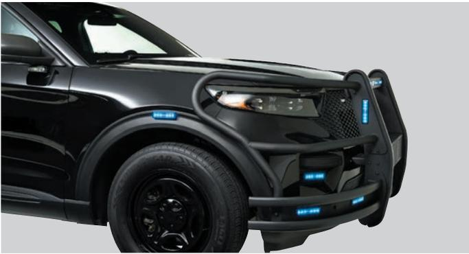
**No drilling is required**, making installation quick and easy. The push bumper features pre-drilled holes to bolt optional lower guard and upper guard.
