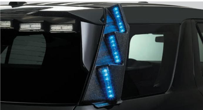
**MicroPulse® Ultra D-Pillar** lighting system is pre-assembled with pre-terminated MPS6U light heads to reduce installation time and is available in (2) tri-color combinations: Red/Blue/White or Red/Blue/Amber.
