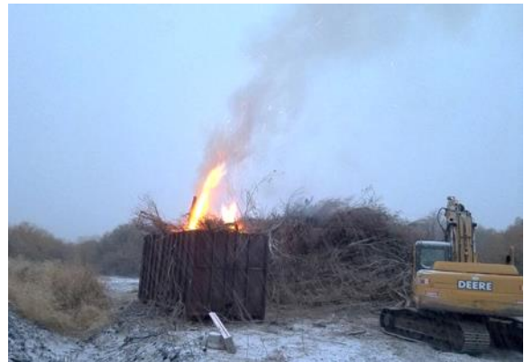
Arborist Brandon Baron makes biochar in a modified 10,000-gallon water tank and a shipping container (Photo: The Tree Service, Burns, Oregon).
