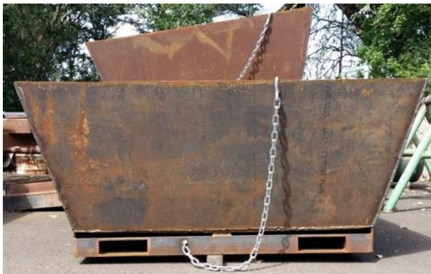
UCC Welding program made heavy duty kilns with fork pockets for easy moving with a tractor or fork lift. One kiln has a spout and tilt mechanism for dumping.
