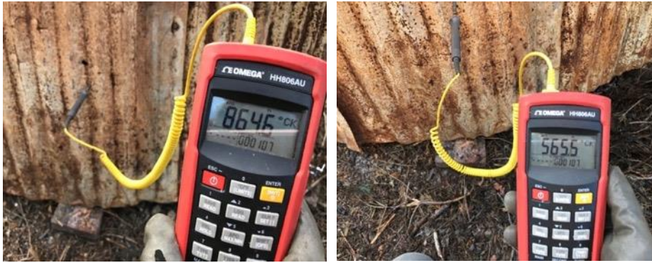
Temperature measurements – Ring of Fire Kiln (shown in degrees Celsius). As the flame front move up during the burn, the finished biochar begins to cool.
