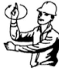
RAISE THE HOOK HOLD THE BOOM
