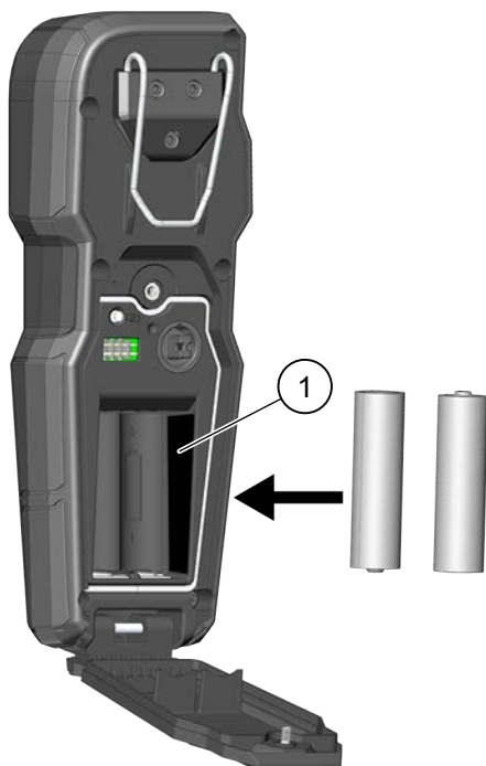
Figure 1. Installing Remote Control Batteries
