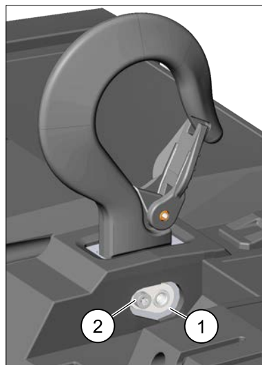
Figure 5. Suspension Pin Retainer/Retainer Screw
