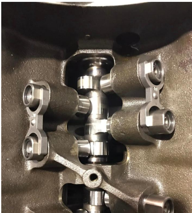
Dog Bone Roller Lifters As Featured In the Ford 5.0 High Output and Link Bar Roller Lifters
