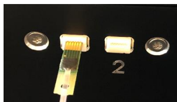
FPC Orientation (copper facing upwards)
