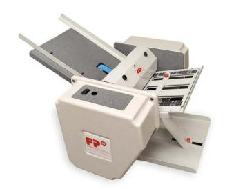
The SFS 1800 offers a powerful solution for processing pressure seal and snap-pack forms.
