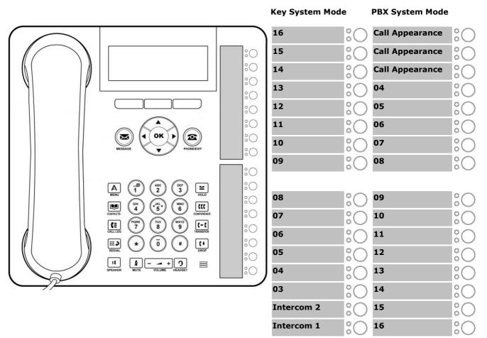
Additional buttons can be added by the addition of up to 3 DBM32 button modules, each module providing 32 programmable buttons. On the button modules, buttons are numbered from top down or bottom up depending on the system mode and then left to right.
