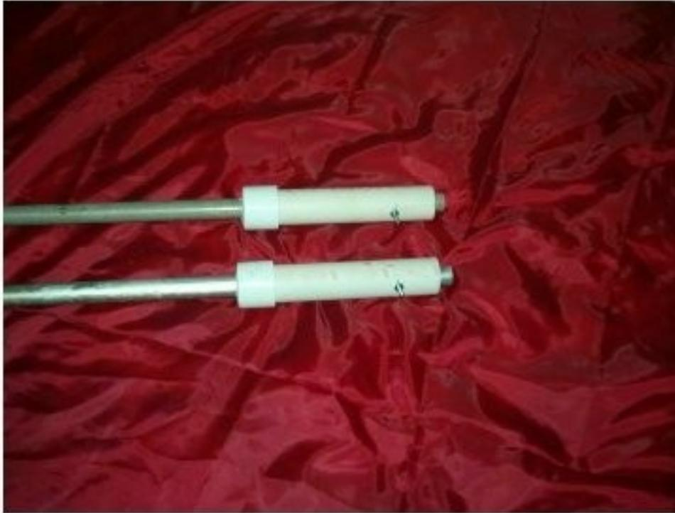
Slide the 0.75-inch diameter tubing inside of the 6-inch PVC. Secure each piece of tubing with the 1.5-inch #6 machine screw putting two "nuts" on the outside. Next slide the "end cap" (with the 0.75-inch hole) over the "long" end of the tubing. Make sure that the cap is securely on the PVC pipe. The small single hole that was drilled on one side of the tubing will extend from the end of the pipe.
