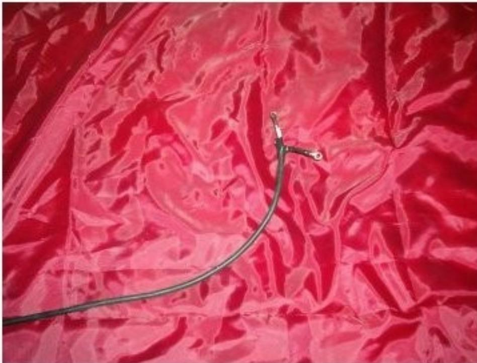
Strip one end of the coaxial cable about 1.5 inches. Make a "hole" in the braid and pull the center conductor through. Remove the insulation from about 0.25-inches of the center conductor. Put a connector on both the center conductor and braid. **SOLDER** the connections! Insulate the braid using black tape including around the coaxial cable as well as along the braid.
