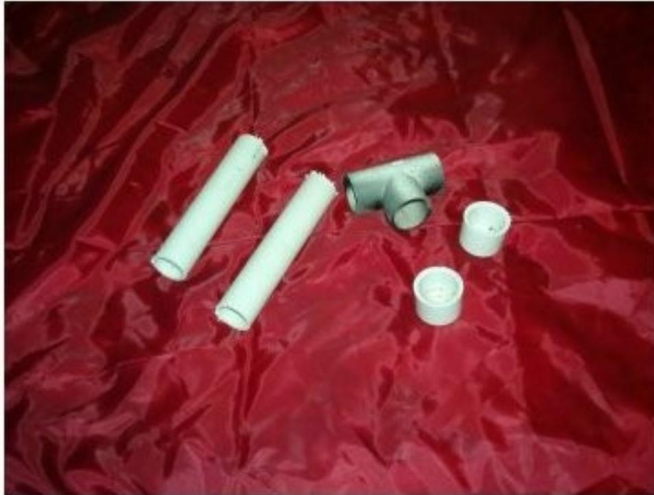
Start by cutting two sections from the 10-foot length of 1-inch PVC schedule 40 (or schedule 80, do NOT use anything with a thinner wall) approximately 6-inches long. Also cut two lengths of the 0.75 outside diameter aluminum tubing 50-inches long and two lengths of the 0.625-inch outside diameter aluminum tubing 12-inches long. The 0.625-inch tubing will just fit inside of the 0.75-inch tubing.
