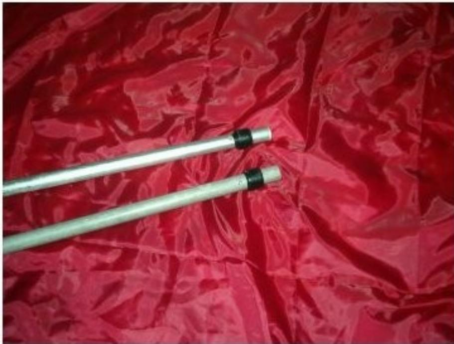
Using the black plastic tape wrap between the two holes that have been drilled in the 0.75-inch diameter aluminum tubing until the wrapped tubing will "just" slide inside of the 6-inch PVC pipe. Do this for both lengths of tubing.
