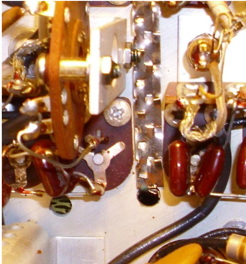
This is the "clip" that needs to be loosened
