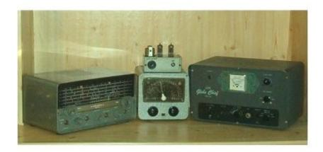
When I upgraded to General Class in October 1959 I added a WRL 755 VFO and a WRL SM-90 screen modulator. The antennas during this time were a 270 foot long true Zepp for 160, 80, 40, 20, and 10 meters. The 15-meter antenna was the home brew 2-element yagi.
