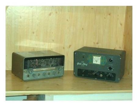
The original equipment at KN9STH (Novice Class call) was a Hallicrafters S-107 receiver and a WRL Globe Chief 90A transmitter. Antennas during this time were a 40-meter dipole and a 15-meter 2-element home brew yagi.
