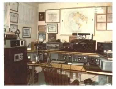
Shortly after moving to the present address in April of 1972 the station looked like this. On the left is a Motorola C53GKB 2-meter FM base station with a separate Motorola 2-meter receiver on top. On top of that is a Motorola Mocom 10 base station that was on the local police department frequency (I was authorized by the police chief to have this station).
