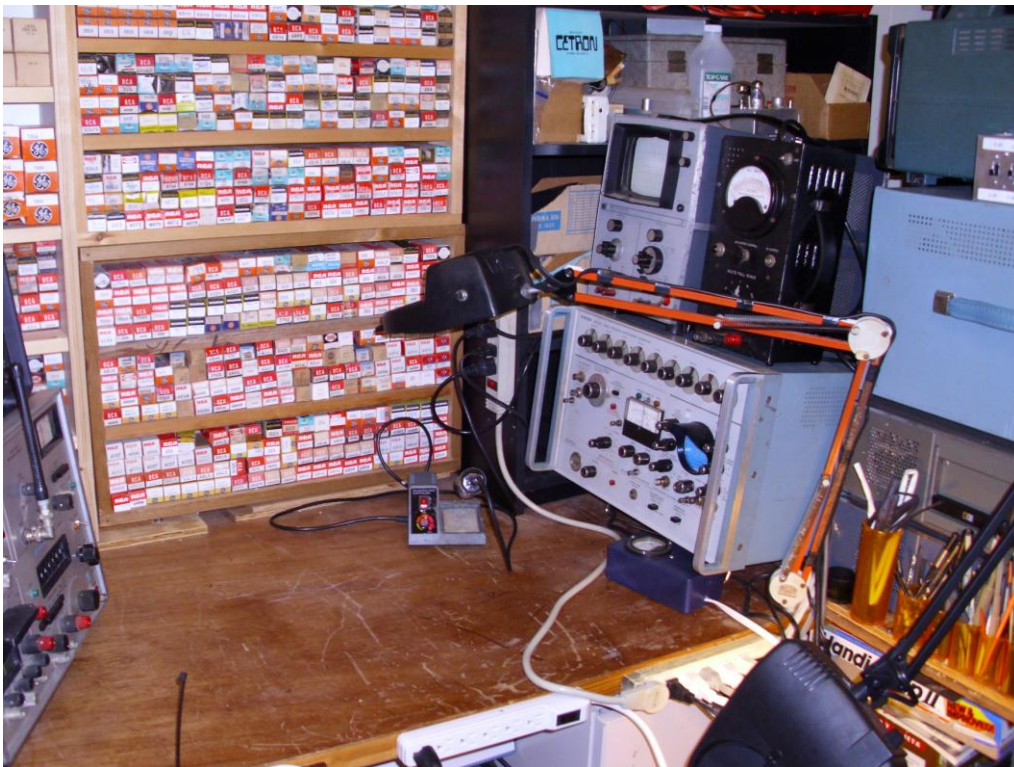
Bench #2 right hand side: Singer-Gertsch FM-10C service monitor. On top HP-600 oscilloscope and Ballantine 300 precision AC voltmeter.
