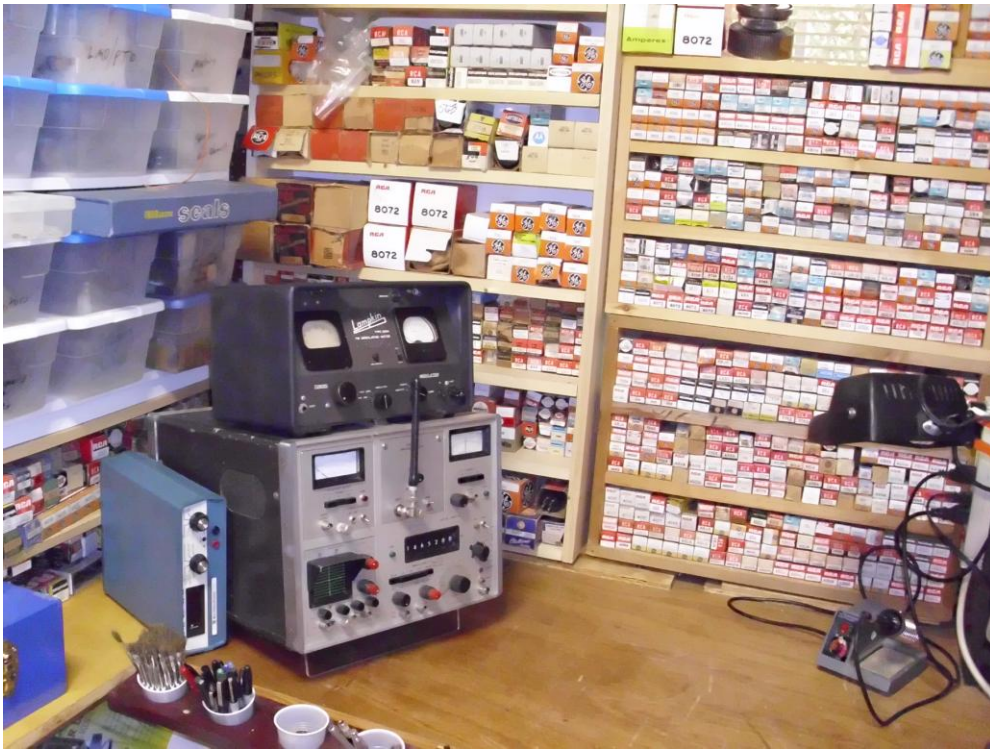
Bench #2 left hand side: Motorola S-1327 service monitor, on top Lampkin 205 deviation monitor, to left Heath DMM
