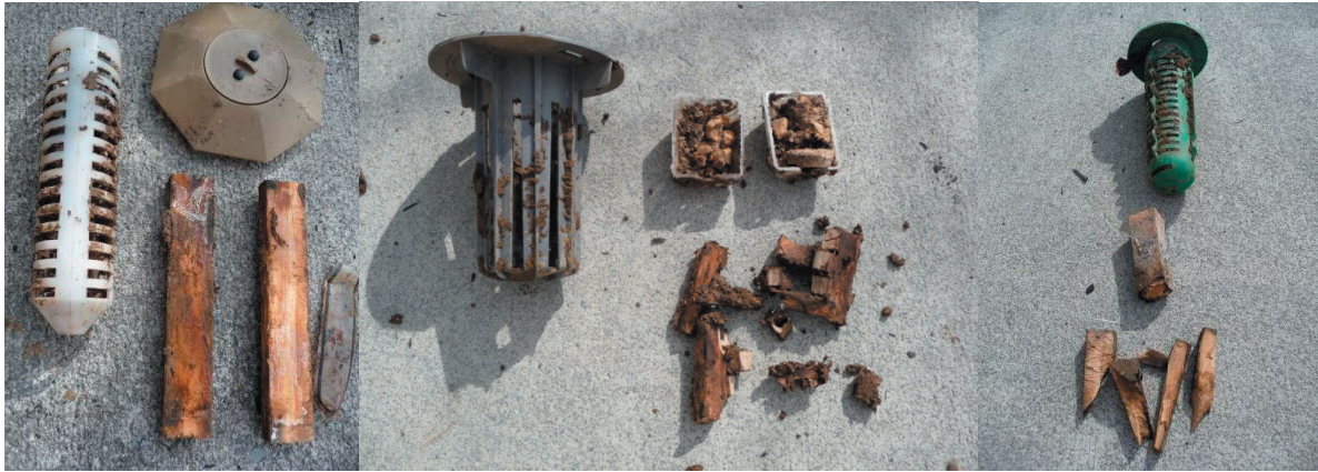
Fig. 1. Fungal decay but no termite activity in commercial termite monitoring stations exposed in Knoxville, TN. From left to right: Halo®; Advance® with cellulose monitor at top and wood below; and Termitrol®.
