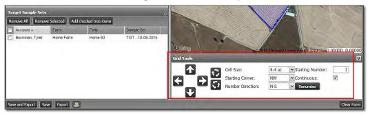
B. Use the grid drop-down menu to view the grid options. Choose the required grid.
