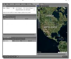
**A.** Click and hold a field and drag into the Fields Account window. Release the mouse to load the field.
