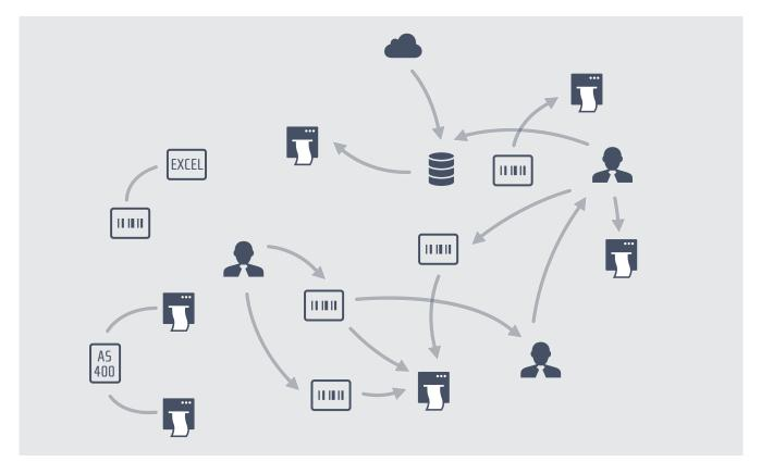
Figure 1: A traditional, decentralized architecture to manage enterprise labeling. With different users and printer types around the world all creating, managing and storing their own label files and accessing different databases and other enterprise systems, what could go wrong?
