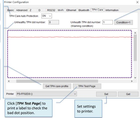
Warning condition, default is "1". "1" means the printer will stop printing if 1 bad dot is detected. If user doesn't care this bad dot, they can click the button [Condition + 1] to extend the limitation.
