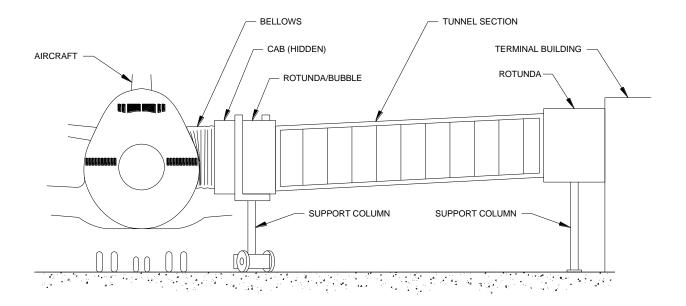
Figure 7. Basic Passenger Boarding Bridge (PBB)
