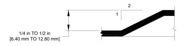
b. SLOPED CHANGE IN ELEVATION UP TO 0.50 in [13 mm]
