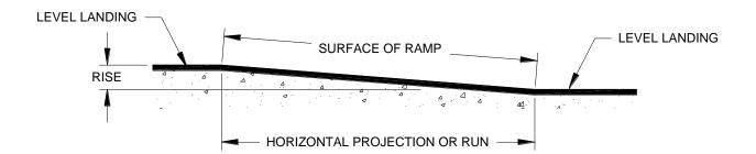
ELEVATION CHANGES GREATER THAN 0.50 in [13 mm] REQUIRE A SURFACE WITH A RECOMMENDED SLOPE OF 1:16 TO 1:20, BUT MUST NOT EXCEED THE FOLLOWING MAXIMUM SLOPES IN THE DIRECTION OF EXPECTED PASSENGER TRAFFIC:
