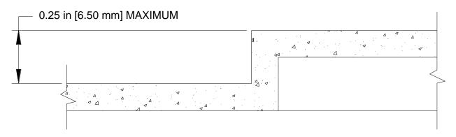
Figure 4. Vertical Change in Level (cross section)
