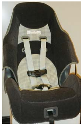
Example of a CRS with Internal Restraint Marketed as a Booster Seat (Approved for use in aircraft during all phases of flight)
