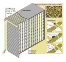
treated with a special adhesive on the airleaving side to prevent blow-off of collected dust. The pleats are generally supported and held in place by wire retainers or welded-wire fabric. Efficiency will range from 25 to 40 percent, according to various manufacturers.
