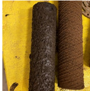
New micron filter on the right side changed after 1 week when the heating season began
