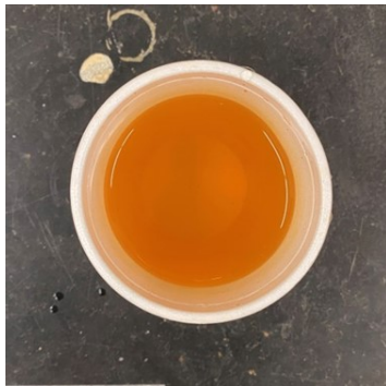
Boiler water that was tested to be acidic – pH of 5.7
